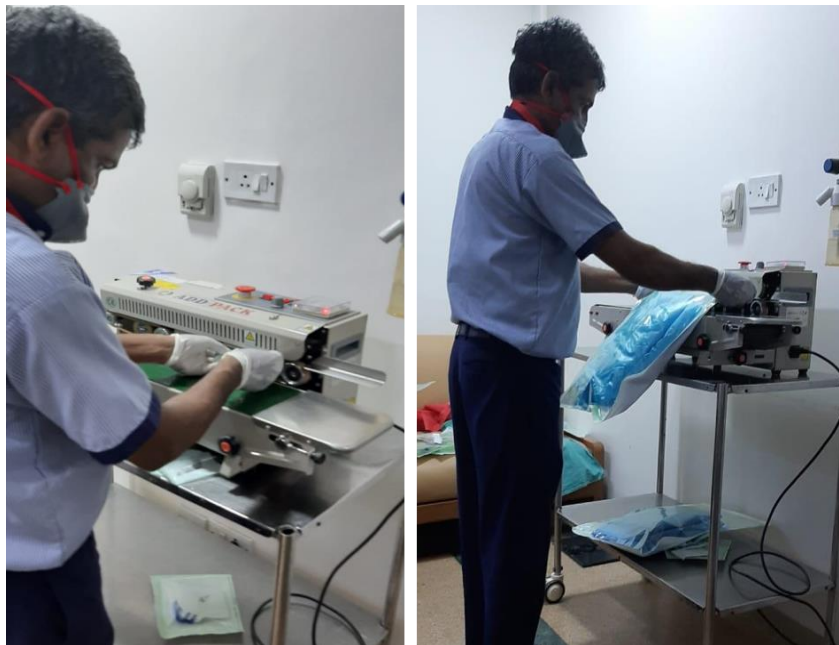
Fig 19- Staff sealing the decontaminated coveralls and N95 masks using sealing machine in Pre-op room (processing area)
