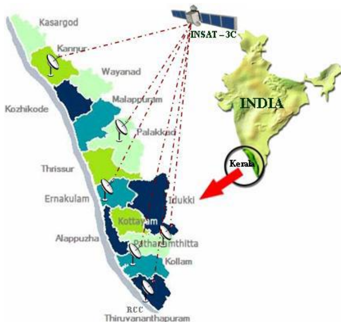
Figure: 3.2.1 VSAT connectivity for RCC and its five nodal centers by using INSAT 3C
